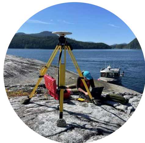
Jessica Heke setting up the GNSS base station at the Cordero Islands
