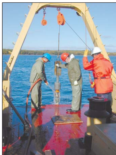
DFO staff use a Lehigh Gravity Core to collect sediment in Sydney Harbour.
