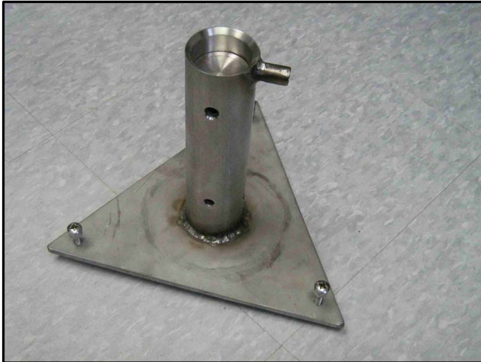
Figure 1. Design of a new overflow apparatus to bring the water level in the evaporation pan to a predetermined level and to redirect the excess water into the stilling well.
