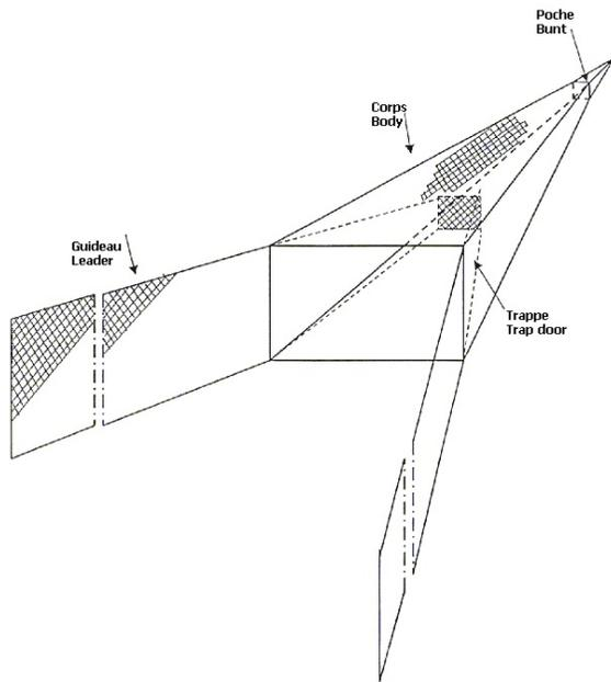
Figure 12. Bag Net (Source: [www.glf.dfo-mpo.gc.ca/fam-gpa/plans/nb/smelt-eperlan\\_2007\\_2011-e.pdf](http://www.glf.dfo-mpo.gc.ca/fam-gpa/plans/nb/smelt-eperlan_2007_2011-e.pdf)).
