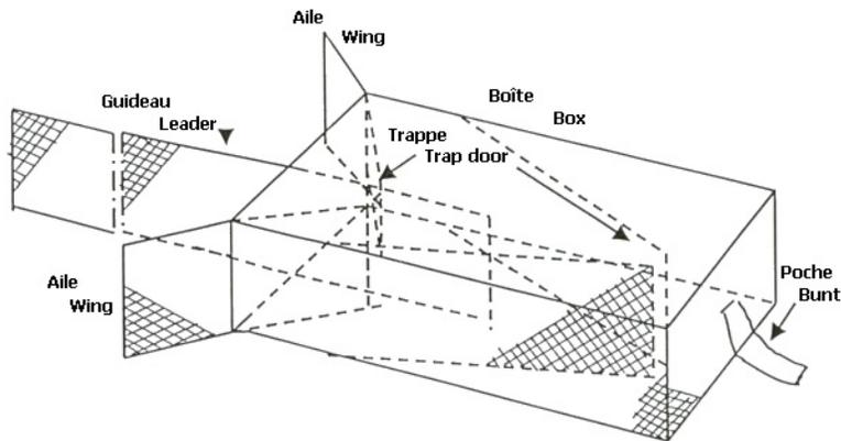
Figure 10. Box Net (Source: [www.glf.dfo-mpo.gc.ca/fam-gpa/plans/nb/smelt-eperlan\\_2007\\_2011-e.pdf](http://www.glf.dfo-mpo.gc.ca/fam-gpa/plans/nb/smelt-eperlan_2007_2011-e.pdf)).
