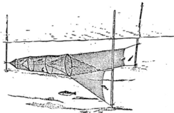
Figure 13. Fyke Net (Source: [www.fao.org/fishery/geartype/226/en](http://www.fao.org/fishery/geartype/226/en)).
