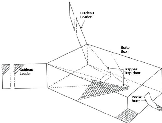
Figure 11. Square Net (Source: [www.glf.dfo-mpo.gc.ca/fam-gpa/plans/nb/smelt-eperlan\\_2007\\_2011-e.pdf](http://www.glf.dfo-mpo.gc.ca/fam-gpa/plans/nb/smelt-eperlan_2007_2011-e.pdf)).
